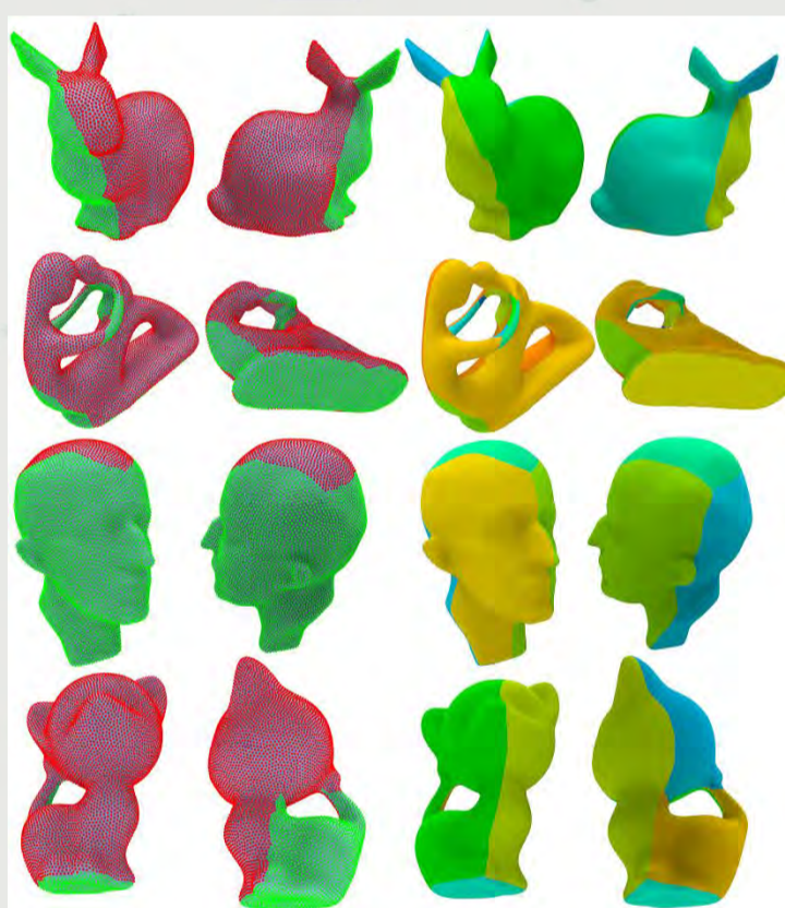
Fig. 4. A gallery of surface decomposition results for 3+2-axis machining. For each model in each row, the first two images show the accessible regions obtained after overlap resolution in two different views; the next two images show the final machinable patches obtained in two views.
